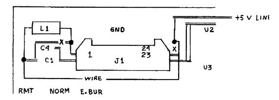
Cut the +5 V line at the shown points (X) Solder the WIRE and/or L1 to the shown points ( )
